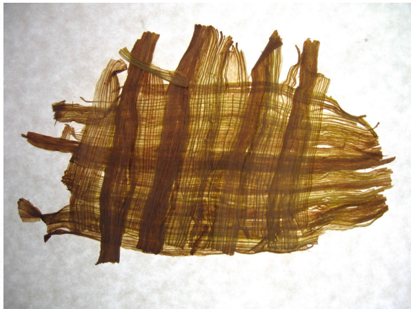
strips layered at 45 degrees with light shining through
